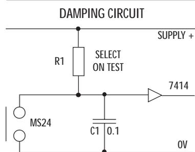
The output of the MS24 may be damped when less sensitivity is required by using a Schmitt trigger device as shown. Lowering the value of R1 (100 ohm min) will reduce the sensitivity of the switch.
