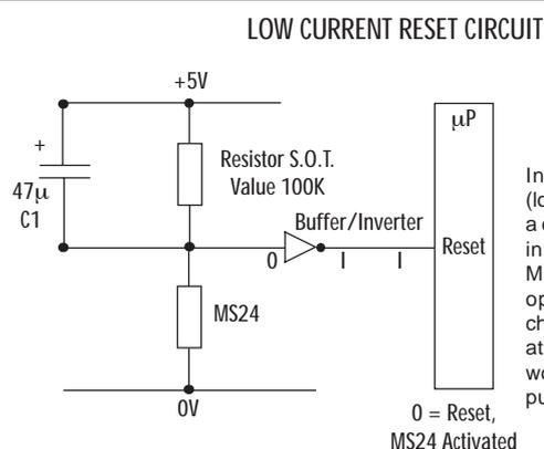
Inverter input held at 0V (logic 0) with no disturbance, a charge is permanently held in C1. With movement the MS24 goes momentarily open circuit allowing the charged capacitor to be seen at the inverter input which would change state giving a pulse to reset.
